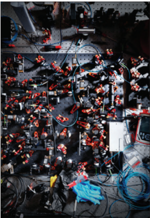
DQ-mat Spokesperson Prof. Piet Schmidt aligning a spectroscopy laser system for highly charged Argon
